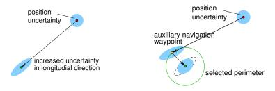
Heading corrections are more precise than odometry
